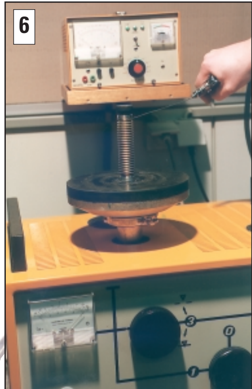
Helium leak testing. Bellows are rejected if leakage exceeds 10^{-8} cm 3 per second.
