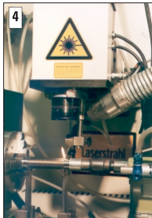
4 Laser welding of bellows to end rings.
