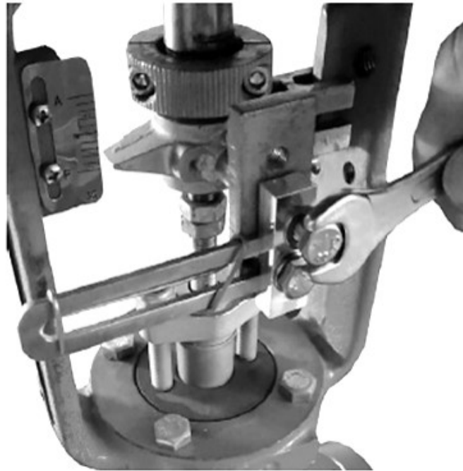
Figure 5-22 Installing the Guide Arm on the Valve Stem
