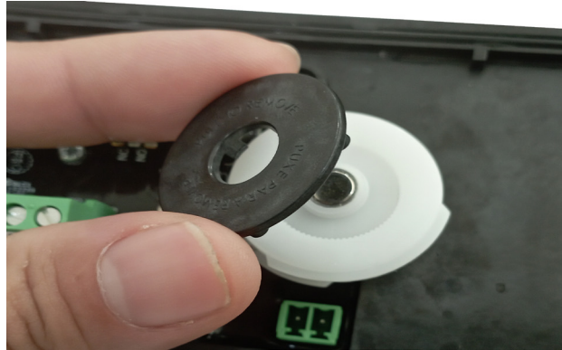
Figure 7-16 Removing the Lock
