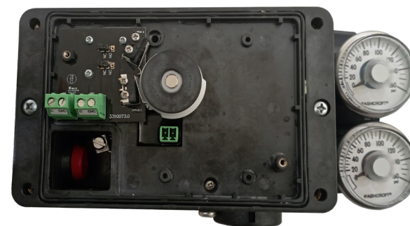
Figure 7-11 View of Jumpers and Cams
