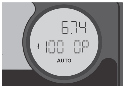
Figure 8-39 Closing Time Stored in Calibration
