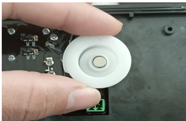
Figure 7-18 Adjusting Lower CAM
