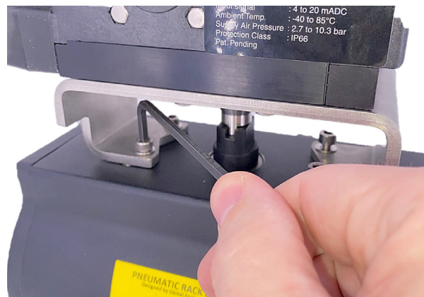
Figure 5-8 Tightening the Bracket Bolts
