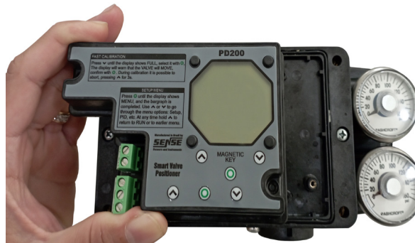
Figure 7-10 Pulling off the Internal Cover
