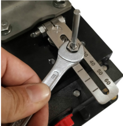
Figure 5-19 Installing the Dowel Pin
