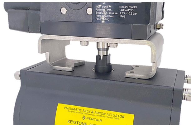
Figure 5-6 Fitting on the Actuator Shaft
