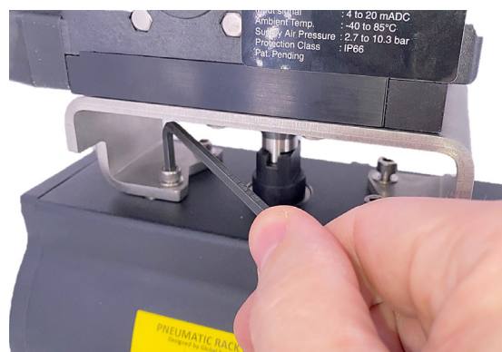
Figure 5-7 Tightening the Bracket Bolts
